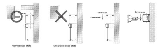
Note: To prevent the wear and the space should be within 1mm between the key and middle of the insert hole.
